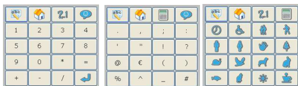
Figure 2. The different aspects of the numpad according to the selected mode (left: number selection, middle: punctuation, right: pre-recorded messages)
