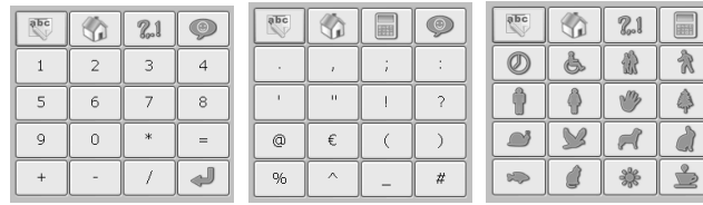
Fig. 3. The three-fold layout of the miscellaneous keypad according to the selected mode (left: number selection, middle: punctuation, right: pre-recorded messages)
